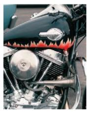
This motorcycle sparkles with chrome plating that was deposited by electrolysis. The shiny, hard coating of chromium is both decorative and a barrier to corrosion. (Syracuse Newspapers/ The Image Works)
