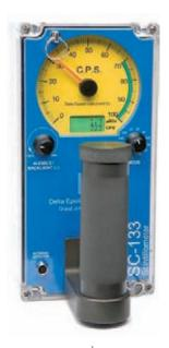
Figure 21.12 | Scintillation **probe.** Energy received from radiations striking the phosphor at the end of this probe is processed
