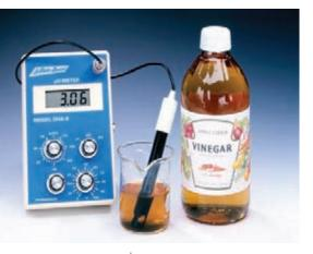
Figure 17.2 | A pH meter. After the instrument has been calibrated with a solution of a known pH, the combination electrode is dipped into the solution to be tested and the pH is read from the meter. (Richard Megnal Fundamental Photographs.)
