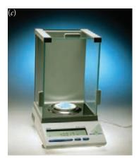
Figure 2.8 | Typical laboratory balances. (a) A traditional two-pan analytical balance capable of measurements to the nearest 0.0001 g. (b) A modern top-loading balance capable of mass measurements to the nearest 0.1 g. (c) A modern analytical balance capable of measurements to the nearest 0.0001 g. (Michael Watson; © 2005 Richard Megna/Fundamental Photographs; Charles D. Winters/Photo Researchers)
