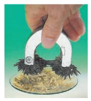
Figure 1.7 | Formation of a mixture does not change chemical composition. Here we see that forming the mixture has not changed the iron and sulfur into a compound of these two elements. The mixture can be separated by pulling the iron out with a magnet. Making a mixture involves a physical change. (Michael Watson)
