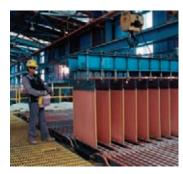
**Copper refining.** Copper cathodes, 99.96% pure, are pulled from the electrolytic refining tanks at Kennecott's Utah copper refinery. It takes about 28 days for the impure copper anodes to dissolve and deposit the pure metal on the cathodes. (Courtesy James Brady)
