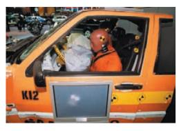
The explosive decomposition of sodium azide releases nitrogen gas, which rapidly inflates an air bag during a crash. (Corbis-Bettmann)
