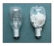
Figure 6.11 | A flashbulb, before and after firing. Fine magnesium wire in an atmosphere of oxygen fills the flashbulb at the left. After being used (right), the interior of the bulb is coated with a white film of magnesium oxide. (Robert Capece)
