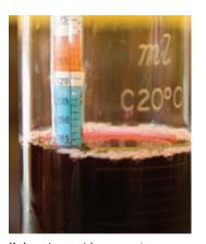
Hydrometer used for measuring sugar content in crushed grapes before fermentation. (WarrenMcConnaughie/ Alamv)
