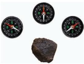
The mineral magnitite like any magnet, is able to affect the orientation of a compass needle. (Visuals Unlimited)
