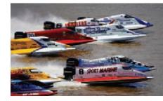
High-speed racing boats often are built with hulls made of Kevlar. Because of the polymer's high strength, the hulls can be made thin, thereby reducing weight and increasing speed. (Martin Bond/ Photo Researchers)
