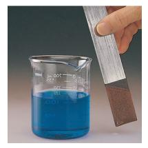
Figure 6.5 | The reaction of zinc with copper ion. (Left) A piece of shiny zinc next to a beaker containing a copper sulfate solution. (Center) When the zinc is placed in the solution, copper ions are reduced to the free metal while the zinc dissolves. (Right) After a while the zinc becomes coated with a red-brown layer of copper. Notice that the solution is a lighter blue than before, showing that some of the copper ions have left the solution. (Michael Watson)
