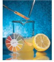
Figure 17.12 | Using a pH test paper. The color of this Hydrion test strip changed to orange when a drop of the lemon juice solution in the beaker was placed on it. According to the color code, the pH of the solution is closer to 3 than to the color for pH 5. (Andy Washnik)
