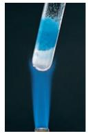
Figure 1.16 | Water can be driven from hydrates by heating. (a) Blue crystals of copper sulfate pentahydrate, CuSO<sub>4</sub>·5H<sub>2</sub>O, about to be heated. (b) The hydrate readily loses water when heated. The light-colored solid observed in the lower half of the test tube is pure CuSO<sub>4</sub>. (Richard Megnal Fundamental Photographs; Michael Watson)
