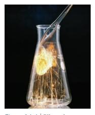
Figure 14.4 | Effect of concentration on rate. Using pure oxygen instead of air, steel wool, after being heated to redness in a flame, burns spectacularly. (© 1993 Richard Megnal Fundamental Photographs)
