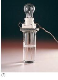
Figure 5.4 | Electrical conductivity of solutions. (a) The copper sulfate solution is a strong conductor of electricity, so CuSO<sub>4</sub> is classified as a strong electrolyte. (b) Neither sugar nor water is an electrolyte, so this sugar solution is a nonconductor. (Michael Watson)
