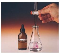
A solution of HCl is titrated with a solution of NaOH using phenolphthalein as the acid-base indicator. The pink color that phenolphthalein has in a basic solution can be seen where a drop of the NaOH solution has entered the HCl solution, to which a few drops of the indicator had been added. (Michael Watson)
