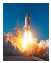
Figure 19.15 | Blastoff of the space shuttle. The large negative heat of formation of Al<sub>2</sub>O<sub>3</sub> provides power to the solid-state booster rockets that lift the space shuttle from its launch pad. (NASA)
