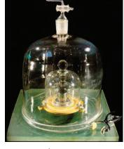
standard kilogram. The SI standard for mass is made of a platinum–iridium alloy and is protected under two bell jars, as shown, at the International Bureau of Weights and Measures in France. Precise copies, called secondary standards, are maintained by many countries.
